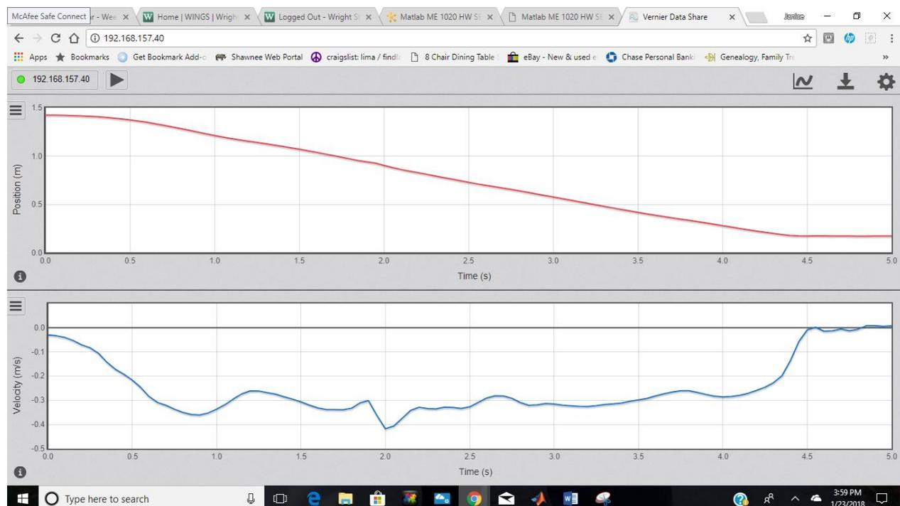
Disappointment: Trials were made both bringing objects toward the detector, and bringing the detector toward the objects. After many trials, even when the position graph is convincingly linear, a more constant velocity graph proved elusive.
