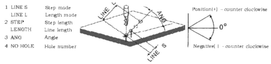
Linear Holes function can simplify the processing multiple holes whose centers are attributed equally on one line.
