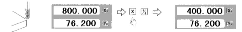
3. Move the maching table until "0.000" is display in X axis window. The position is the work-piece's center
