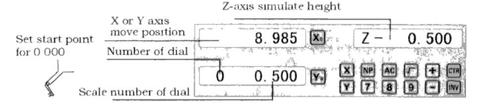
Z-axis simulate height = Number of dial x Z axis Dial + Scale number of dial
