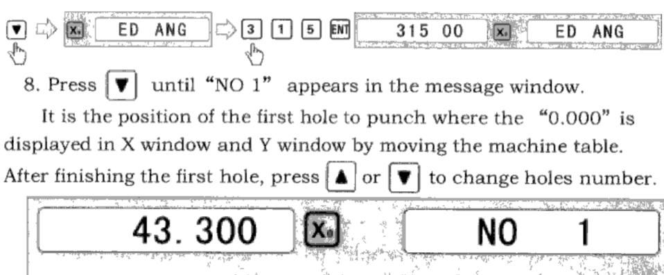
9. After processing all holes, press 🙀 to return normal display.
