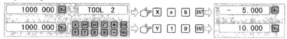
Step 4: Press to continue to input the data of next tool. By pressing number and the key [INT], the operator can directly input the special tool data. Press [TOOL] to quit.
