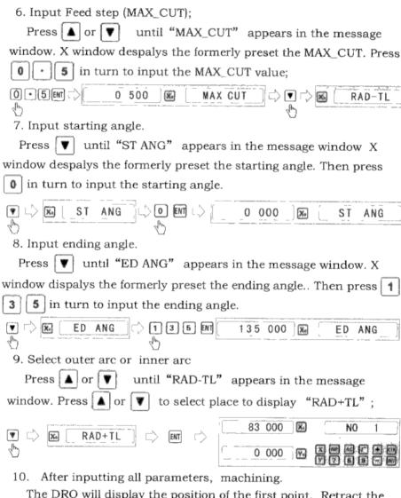
The DRO will display the position of the first point. Retract the axes until the displays read 0.000, Machine the Arc point by point in accordance with the display. After finishing the position of the first point, press or to change position point.
