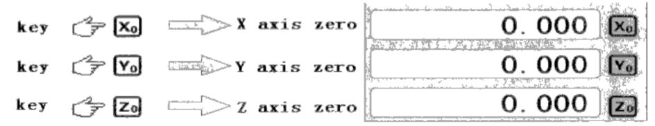
Press AC +  $X_0$  or  $Y_0$  or  $Z_0$  will be return to the original data before the reset.
