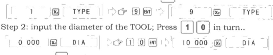
Step 3: Press 🔻 to the machining Mode.
