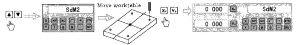
3. Set the point sdm1 as the datum of SDM 3. Move the machine worktable to x = -60.000, y = -45.000. Then proess  $X_0$   $Y_0$ .
