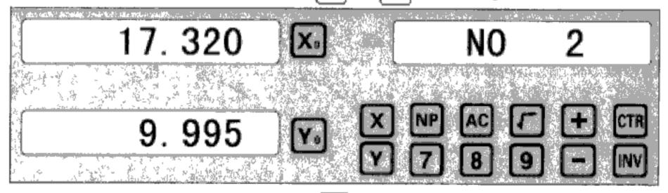
7. After processing all holes, press 🙋 to return normal display.
