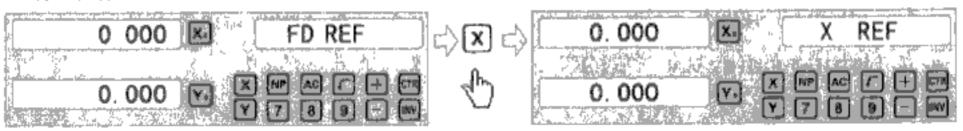
4. Move the machine table .The buzzer sounds when RI is searched, then X window stops flashing and displays the value of the current position .the DRO returns normal display state. Then message window displays "FIND\_X" .
