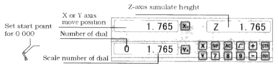
Z-axis simulate height = Number of dial x Z axis Dial + Scale number of dial
