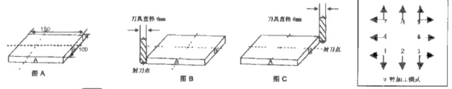
Step1: press to enter the TOOL compensation Function. then the message window display "TYPE" .Press 9.
