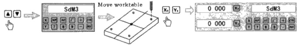
4. Set the point sdm1 as the datum of SDM 4. Move the machine worktable to x = -60.000, y = 45.000. Then proess  $X_0$   $Y_0$ .
