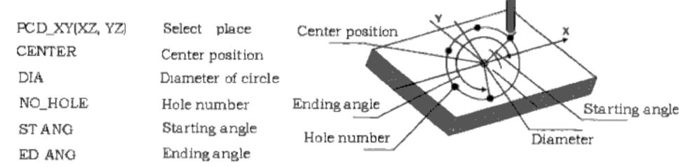
The postion of the hole center are calculated automatically after input all parameters. Press ( or ) to choose the hole No. and move the machine table until the "0.000" appears in X window, Y window, Z window. It is the position to process a table.
