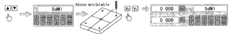
2. Set the point sdm1 as the datum of SDM 2. Move the machine worktable to x = 60.000, y = -45.000. Then proess  $X_0$   $Y_0$ .
